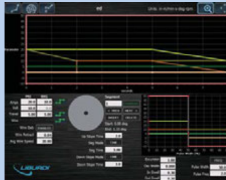
Schedule Editing Screen - Load and save schedules, set weld parameter values and view a graphical representation of the weld sequence, rotary position and pulse shape.
