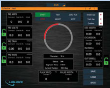
Run Weld Screen - Welding telemetry and rotary position are displayed in real time.
