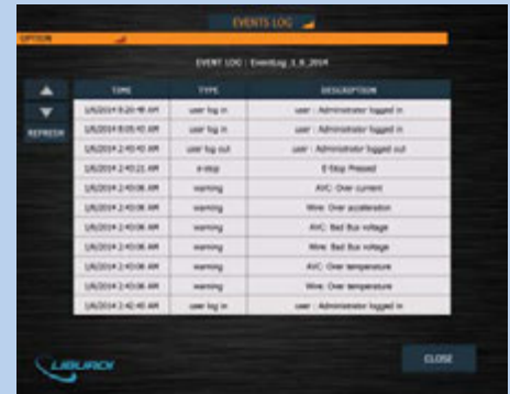
Event Log Screen - Review system events like alarms, user login/logout and emergency stops.
