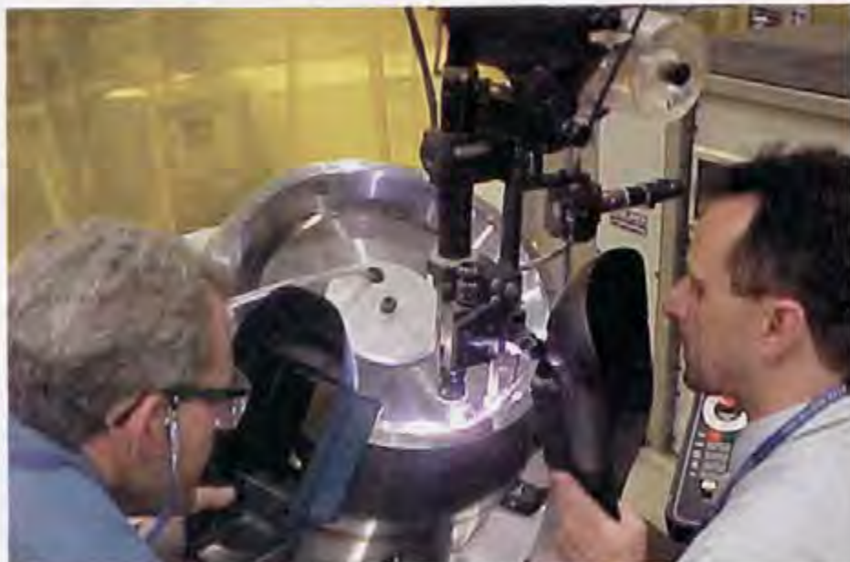
Automated arc welding of a case assembly at Pratt & Whitney Montreal
