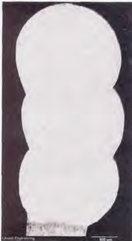
HPC blade welded by PAW with cold wire feed (Titanium).
