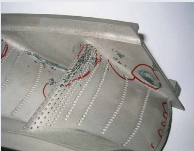
HPT NGV pre-repair: thin wall, oxidized burnt metal loss.
