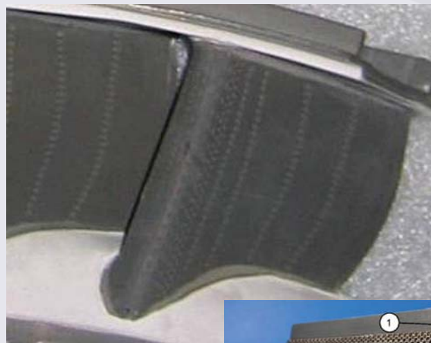
HPT NGV after LPM® Reconstruction Repair
