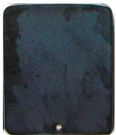
400 hrs some stains no pitting
