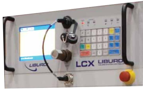
LCX™ allows you to work seamlessly with a variety of industry power supplies, including our own line. In conjunction, the LCX™ is fully compatible with Liburdi Dimetrics Gold Track pipe welding systems.
