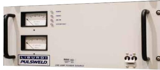
The Puls weld P200-006 current source is designed for use in Variable Polarity configurations greater than 100 amps. This unit is designed to accept DC power from a Puls weld Power Console, such as a T400.
