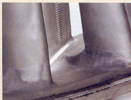
Figures 4, 5: Frame 7EA Nozzle after 24,000 hours service repaired with a standard weld (left) and an advanced powder metallurgy process (right)
