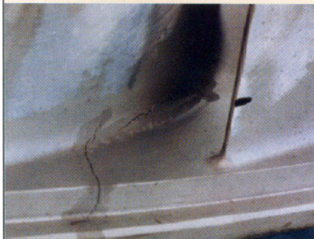
Figures 4, 5: Frame 7EA Nozzle after 24,000 hours service repaired with a standard weld (left) and an advanced powder metallurgy process (right)
