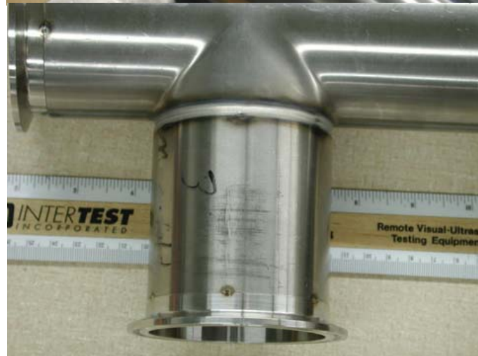
Completed pull tee
