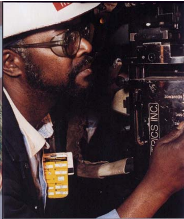
Above: Welder Mike Howard operates an automatic pipe welding machine aboard Reagan . A nuclear pipe welder with 18 years of experience, Howard was part of a welding team who achieved unprecedented success during construction by welding all shipboard main coolant piping joints on Reagan without a single defect.
