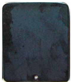
400 hrs some stains no pitting
